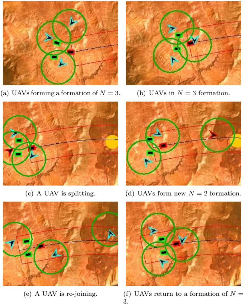
Figure 10: Simulation of three UAVs executing the convoy protection algorithm. ( $N$  is the number of UAVs along the UGV convoy.)
