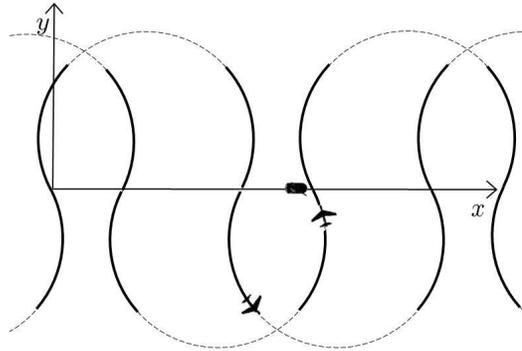
Figure 7: Example of using two UAVs to provide continuous convoy protection using the proposed strategy. In this figure, the dashed curves are the paths of the UAVs, the solid curves are the segments of the paths in which convoy protection is provided. In this case, every time one UAV exits the convoy circle, the other UAV is inside the convoy circle. This is always true if  $N = \lceil \frac{\beta}{\gamma^*} \rceil = 2$  and the times when the UAVs synchronize with the UGVs are spaced out.
