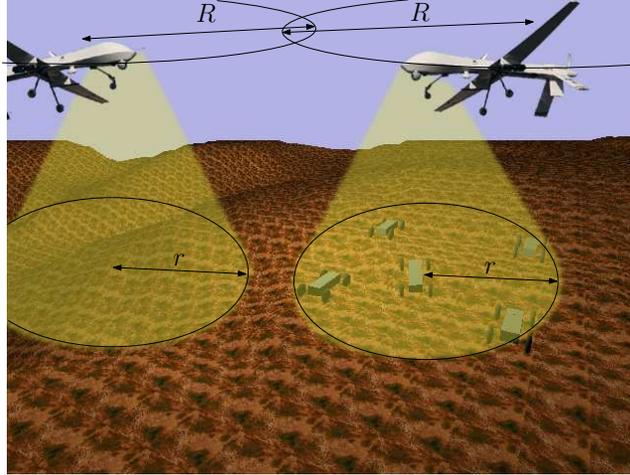
Figure 1: UAVs providing convoy protection to UGVs. The UAVs are assumed to be kinematically restricted by their minimum turning radius  $R$ . The sensors on board the UAVs also have limited range and are assumed to be able to observe a disk of radius  $r$  on the ground.
