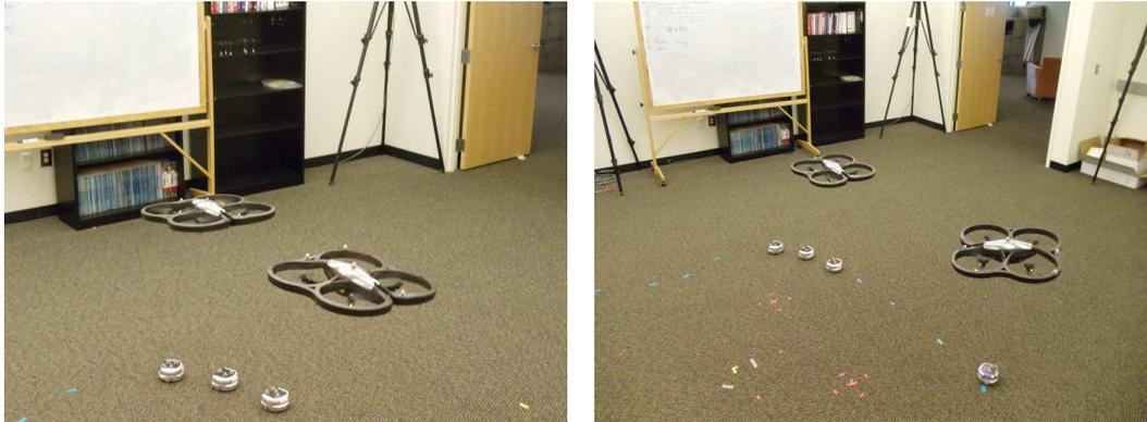
(a) Two UAVs protect the convoy while maintaining the spacing from one another. (b) One UAV is dispatched to visit a threat, while the other remains with the convoy.
