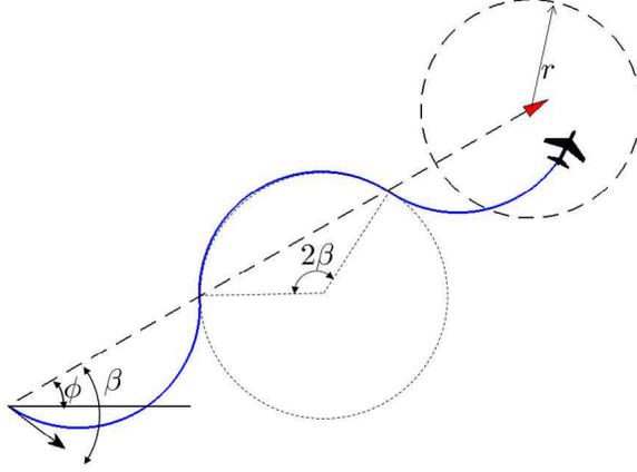
Figure 5: Example trajectory of a UAV providing convoy protection for the UGVs with the proposed control strategy. The solid curve is the path of the UAV. The dashed line is the path of the UGVs. The dashed circle is the convoy circle. The angle of the circular arc for each motion primitive is  $2\beta$ . In this case,  $\beta \in [0, \frac{\pi}{2}]$ .
