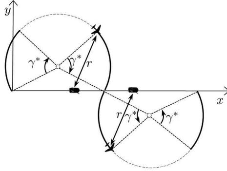
Figure 6: For each execution of one motion primitive, there are two segments of the path corresponding to two circular arcs of angle  $\gamma^*$ , so that the distance between the UAV and the UGVs is less or equal to  $r$  when the UAV is on these segments. In this figure, the dashed curve is the path of the UAV, the solid curves are the segments of the path in which convoy protection is provided. The UAV and the convoys are drawn at the times when the UAV enters and exits these segments.
