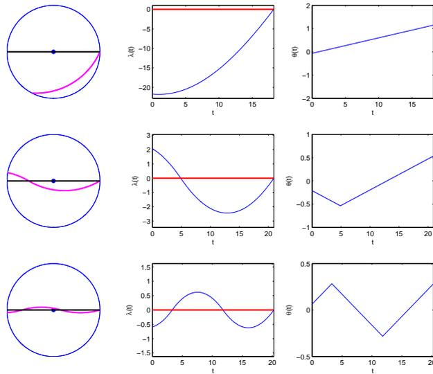
Figure 2: A number of COTs are plotted for different exit angles  $\theta_T$  resulting in different number of switchings. The left plots are the COTs in  $x$ - $y$  plane, the middle plots are the costates  $\lambda_3$  and the right plots are the angles  $\theta(t)$ . The first, second and third row correspond to the cases when this is 0, 1 and 2 switchings, respectively.
