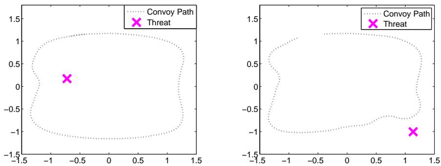
(a) The original intended path taken by the convoy, corresponding to Figures 12(a) and 12(b). (b) The recomputed path of the convoy upon being informed of a persistent threat, corresponding to Figure 12(c).
