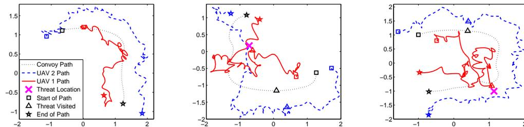
(a) Two UAVs perform convoy protection on UGVs. (b) A UAV is dispatched to clear a non-persistent threat. (c) A UAV identifies a persistent threat and the convoy re-plans its path.
