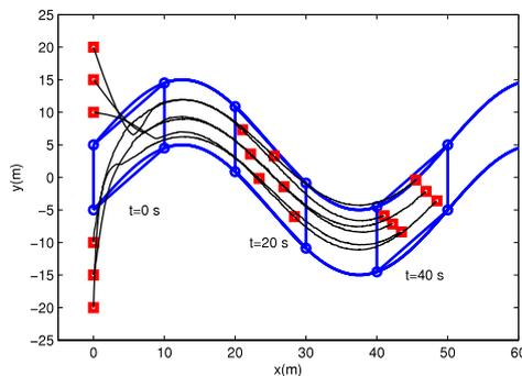
**Fig. 10.** Trajectories of the agents using (13) under a fixed directed network topology in the 2D space. Circles denote the positions of the dynamic leaders while the squares denote the positions of the followers. Two snapshots at  $t = 20$  and  $t = 40$  s show that all followers converge to the dynamic convex hull formed by the dynamic leaders.
