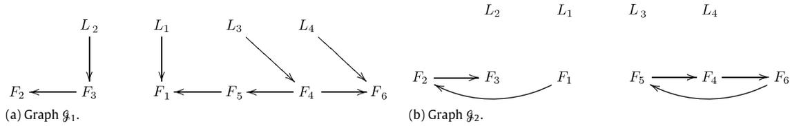
**Fig. 8.** Switching directed network topologies for a group of agents with four leaders and six followers. Here  $L_i, i = 1, \dots, 4$ , denote the leaders while  $F_i, i = 1, \dots, 6$ , denote the followers.
