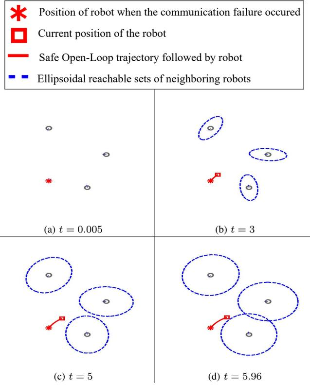
Fig. 4: The safe time horizon represents the longest time duration for which the robot lies outside the ellipsoidal reachable sets of other robots. Thus, the robot experiencing communication failure can execute its last received velocity command for the corresponding safe time horizon and remain safe. Beyond this, the robot stops moving.
