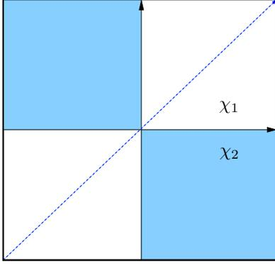
Fig. 3. State space of Example 3. The blue line represents the “direct controllability” subspace of  $(A(2), C(2))$ , which intersects  $\chi_2$  at 0.
