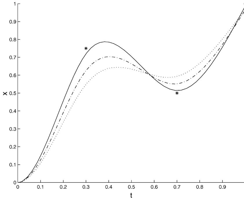
Fig. 1. A smoothing spline with different smoothing parameters,  $\rho$ , is shown. The parameters are 1/10000 (solid), 1/2000 (dash-dotted), and 1/1000 (dotted). The  $\tau_i$ 's are all equal to one, and the stars correspond to the different waypoints. The underlying second order system was given by  $\ddot{x} = u$  and  $y = x$ .
