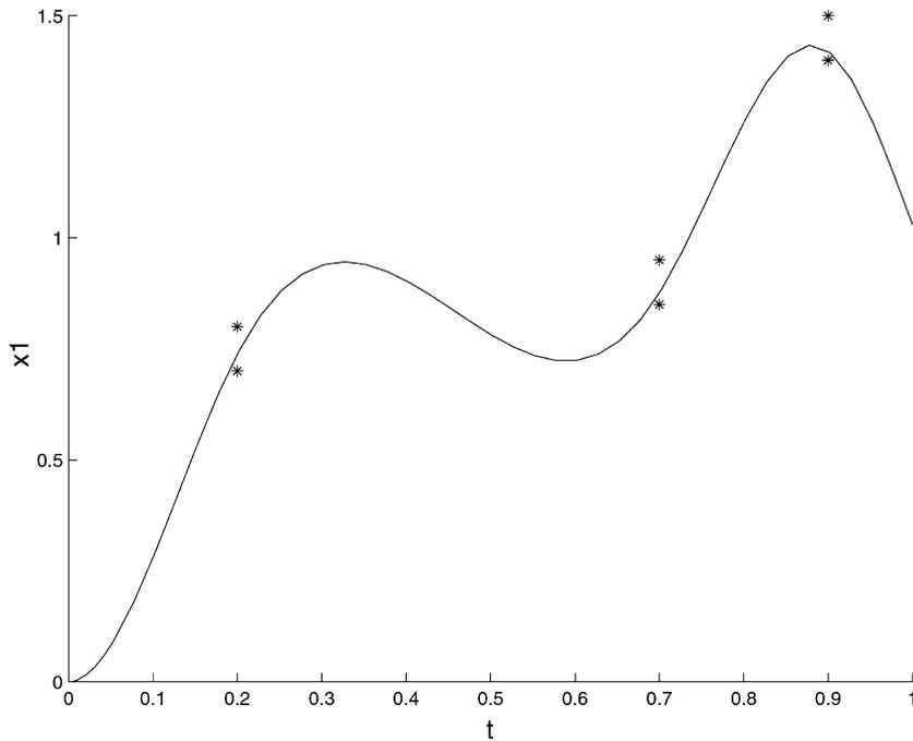
Fig. 3. Interpolating through intervals while penalizing deviations from the mid points of the intervals. Here, a second order system with both eigenvalues equal to  $-1$  was used to produce the scalar output  $y = x_1$ , with  $\dot{x}_1 = -x_1 + x_2$ ,  $\dot{x}_2 = -x_2 + u$ .
