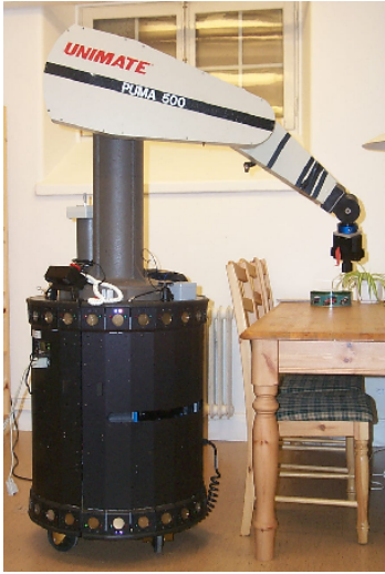
Figure 1: The Nomad XR4000 platform with a Puma560 arm on top on which the MMCA is implemented.
