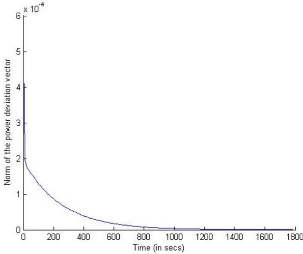
Fig. 8: Plot of power deviations ( $L = 560$ , optimization procedure = Nesterov's accelerated descent)
