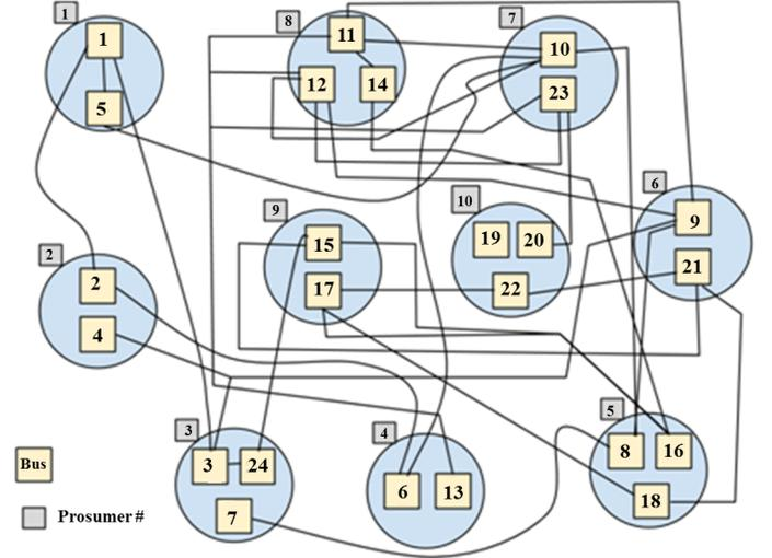
Fig. 5: Schematics of the cyber-physical grid of the prosumer-based IEEE 24-bus system
