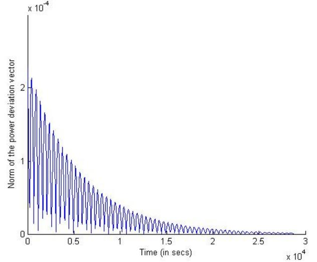
Fig. 9: Plot of power deviations ( $L = 3600$ , optimization procedure = steepest descent)
