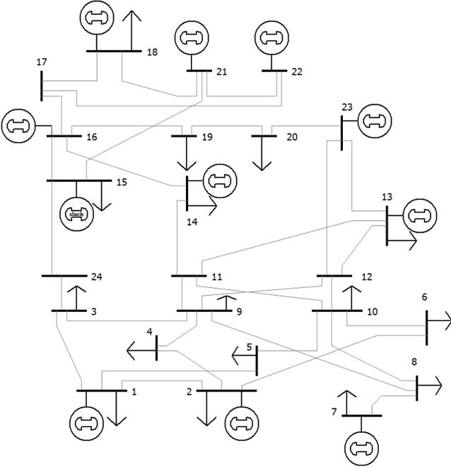
Fig. 4: Schematics of the power grid of the IEEE 24-bus system [20]
