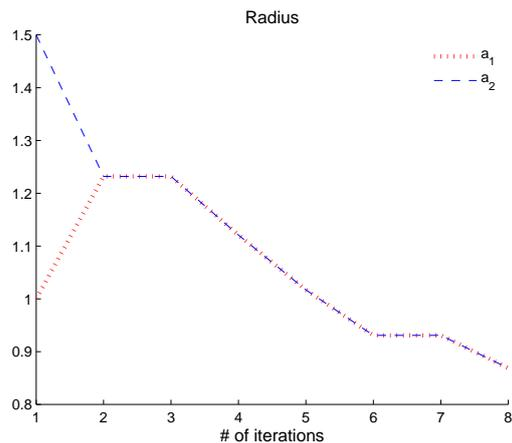
Fig. 5. Change in  $a = (a_1, a_2)^T$  as a function of the number of gradient descent iterations in Algorithm 3.2.  $a_1$  is the radius of the *obstacle-avoidance* switching surface,  $a_2$  is the radius of the *go-to-goal* switching surface.
